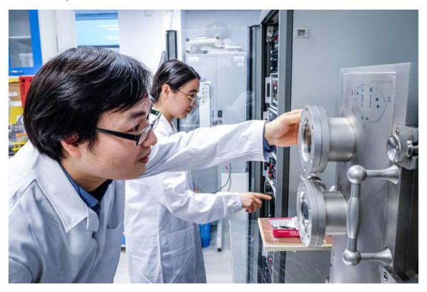
The researchers used a vacuum evaporation system to synthesize the remaining layers of the perovskite solar cell, a method commonly used for the fabrication of perovskite solar cells. Credit: NTU Singapore.
